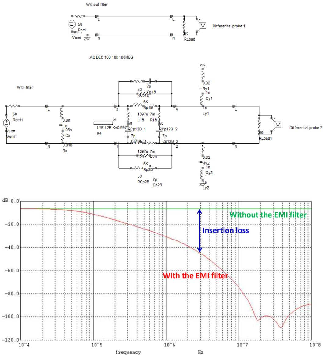
Circuit model for the computation of insertion loss of the filter in case of CM disturbance (IL\_CM\_noise\_real.sch). Comparison with the results of question 5 shows that the IL is similar to the ideal model version up to 350 kHz. Above this frequency, the CM inductance of the choke is no more a pure inductance. As shown in Fig. 5-32, a lossy behaviour appears and the self-resonance arises at nearly 1 MHz. Due to the stray components of the passive devices, the IL does not exceed 50 dB.
