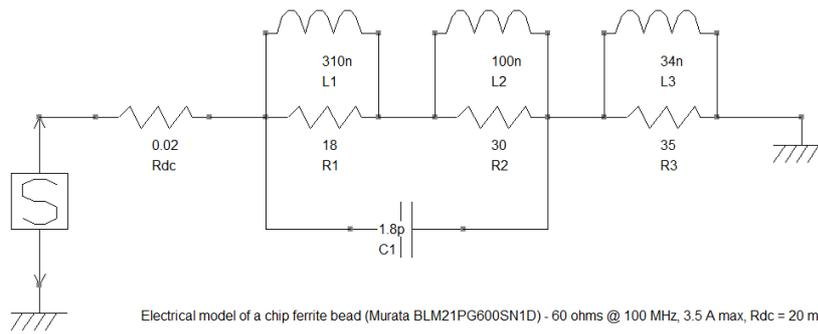
Electrical model of a chip ferrite bead (Murata BLM21PG600SN1D) - 60 ohms @ 100 MHz, 3.5 A max, Rdc = 20 mohms
