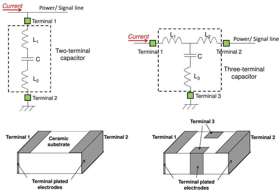
1. Initially, we assume that lead inductances are identical in two- and three-terminal capacitors and equal to  $L$ . What is the ratio between the equivalent series inductance (ESL) of two- and three-terminal capacitors?
